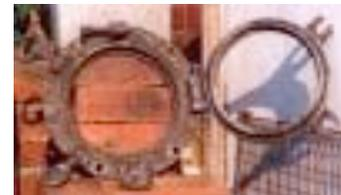
**Figure 2 Port Hole after Acid Treatment**
